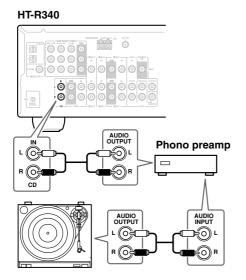
■ Turntable with an MC (Moving Coil) Cartridge An MC head amp and phono preamp are necessary to connect a turntable with an MC (Moving Coil) cartridge.
